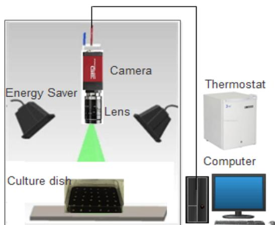
**Fig. 1:** Demonstration diagram of the self-developed system
