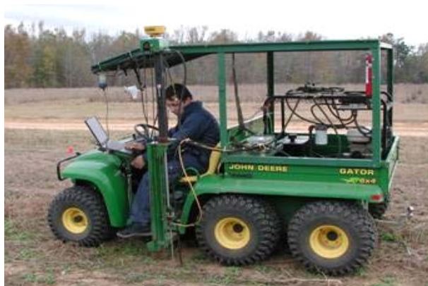
Fig. 2. The control system for variable-depth tillage operations
