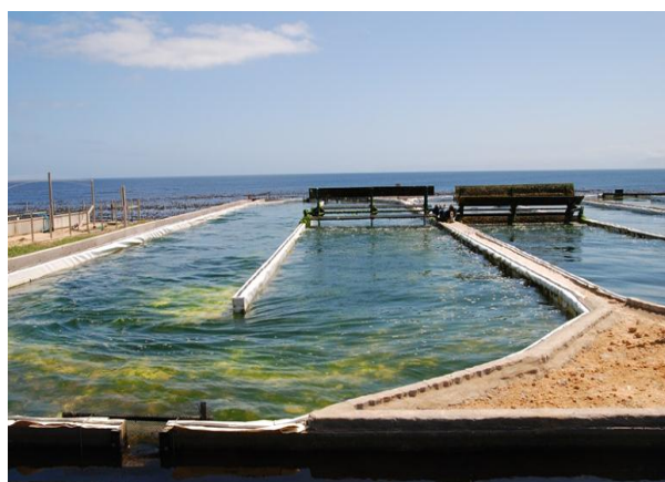
Fig. 1: Flow-through, paddle-wheel raceways are the preferred method for growing Ulva
