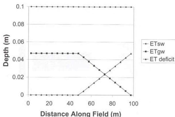
**Fig. 5. Irrigation performance with and without a water table contribution along the field for first irrigation with 21-day irrigation interval and complete irrigation at the downstream end**
