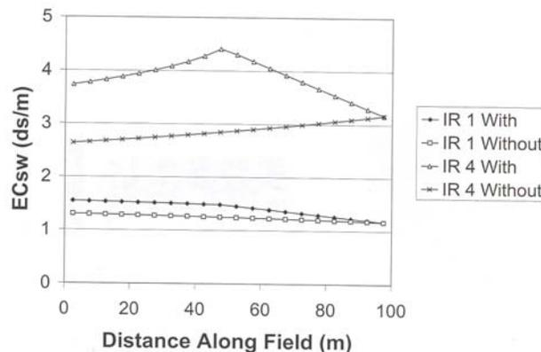
groundwater contribution, EC<sub>sw</sub> is nearly 1.5 dS/m from the up-stream end to the middle of the field and thereafter decreases linearly to 1.2 dS/m at the down-stream end. With groundwater contribution, EC<sub>sw</sub> is higher, because Setgw is added to the soil water salt. For the fourth irrigation without
