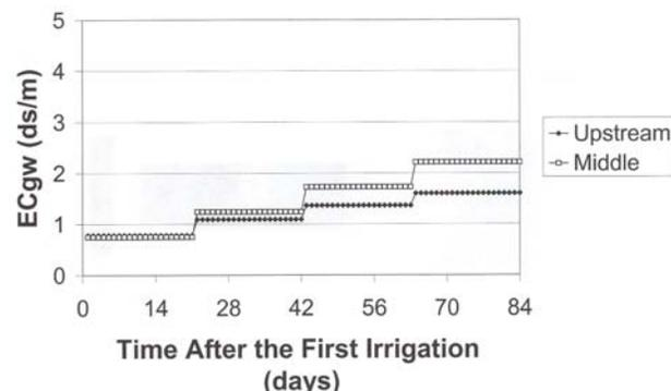
differences increase from irrigation to irrigation throughout the irrigation season. During the first 14 days the difference is constant, because up to that time there is enough soil water to satisfy the ET demand and it evapoconcentrates at the same rate in both cases. Thereafter, salty groundwater contributes to the ET demand and therefore soil water concentration increases in the groundwater contribution case.
