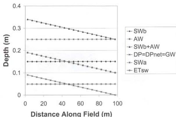
**Fig. 3. Irrigation performance with and without a water table contribution along the field for first irrigation with 7-day irrigation interval and complete irrigation at the downstream end**
