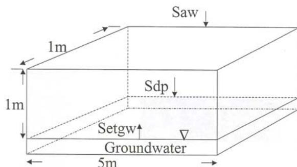
**Fig. 2. Water budget components for first irrigation with 7-day irrigation interval and complete irrigation at the downstream end**
