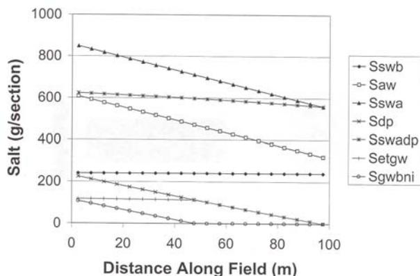
**Fig. 7. Salt budget for fourth irrigation for 21-day irrigation interval**
