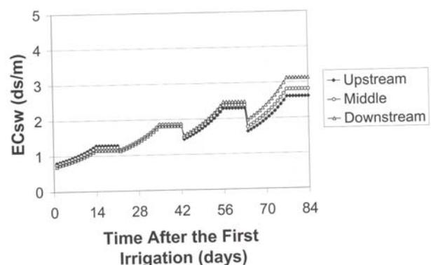
**Fig. 12. Groundwater EC with groundwater contribution with time at upstream and middle section for 21-day irrigation interval**
