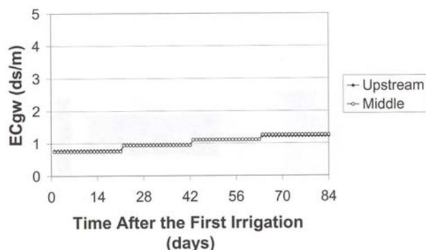
**Fig. 14. Field average soil water EC with and without groundwater contribution with time for 21-day irrigation interval**
