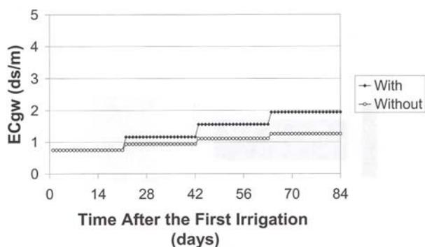
ET demand and groundwater has no contribution to the ET demand. After water application, as shown in Fig. 16, EC<sub>sw</sub> increases with time, because soil moisture declines with time due to root water extraction for all three irrigation intervals, while soil salt remains constant (for 7 & 14 days irrigation intervals) or even increases (for 21 days irrigation
