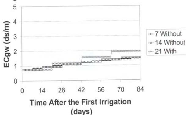
intervals, without groundwater contribution, field-average EC<sub>gw</sub> is the same as 7 and 14 days irrigation intervals (not shown). Without groundwater contribution, the field-average EC<sub>gw</sub> is nearly the same for all three irrigation intervals.
