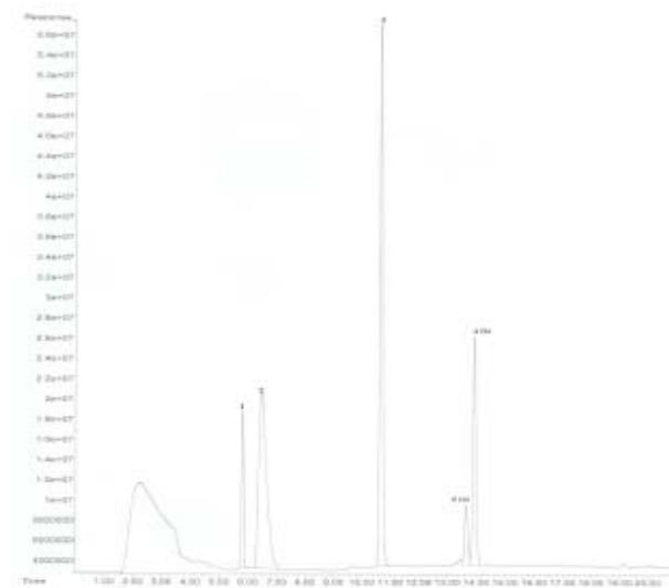
**Fig. 4. Separation of four pesticides in wheat grain fortified at 0.1 mg/kg quantifying on a 30 m HP-5 MS capillary column, Peaks: 1. malathion, 2. chlorpyriphos, 3. bifenthrin and 4. permethrin (a, b)**
