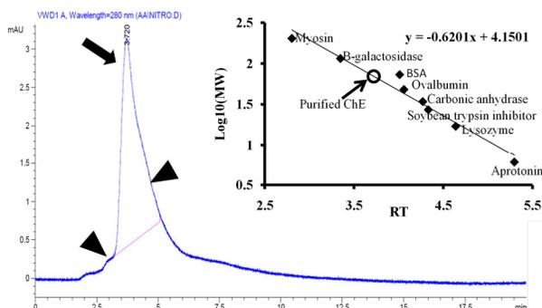
**Fig. 3:** Profile of purified ChE from *P. javanicus* on Zorbax GF-250 column attached to HPLC
