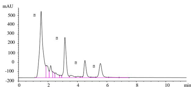
**Fig. 1:** High-performance liquid chromatogram of the root extracts. The mobile phase was methanol–water (90:10), and the detection wavelength was 214 nm
