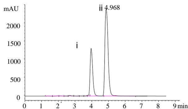
**Fig. 3:** High-performance liquid chromatogram of peak 3. The mobile phase was methanol–water (90: 10), and the detection wavelength was 340 nm
