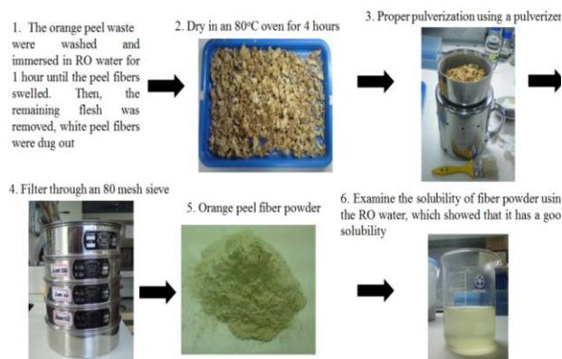
**Fig. 1:** Procedure for preparing OPFP
