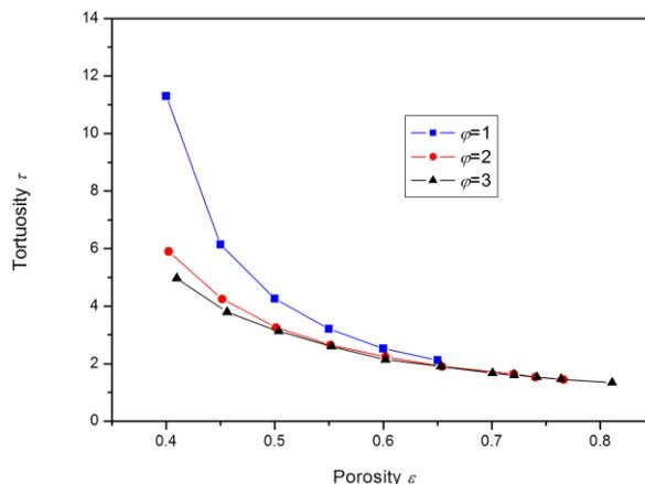
**Fig. 2:** Effect of porosity  $\varepsilon$  on tortuosity  $\tau$  with different  $\phi$
