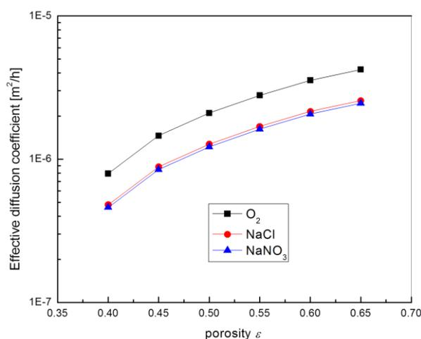
**Fig. 3:** Effect of porosity  $\varepsilon$  on effective diffusion coefficient of NaCl, O<sub>2</sub> and NaNO<sub>3</sub>
