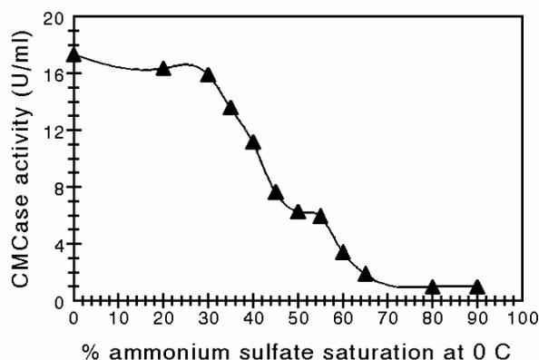
**Fig. 5. Effect of ammonium sulfate on activity of CMCases**
