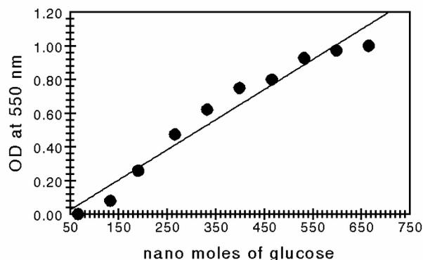
**Fig. 3. Standard curve of cellulose estimation and determination of molar extinction coefficient**
