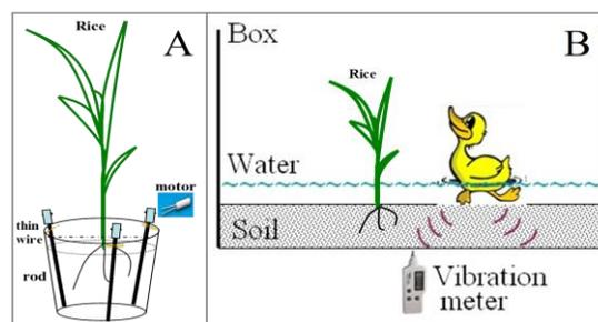
**Fig. 1:** Vibration mechanism (A) composed of vibrating motor, glass rod and thin wire; the glass rod was fixed onto the top of inner wall by thin wire. The motor was fixed on the glass rod using scotch tape. Three glass rods were distributed at a  $120^\circ$  angle; Vibration intensity (B) was measured on ducks using a vibration meter in a box with paddy soil and water
