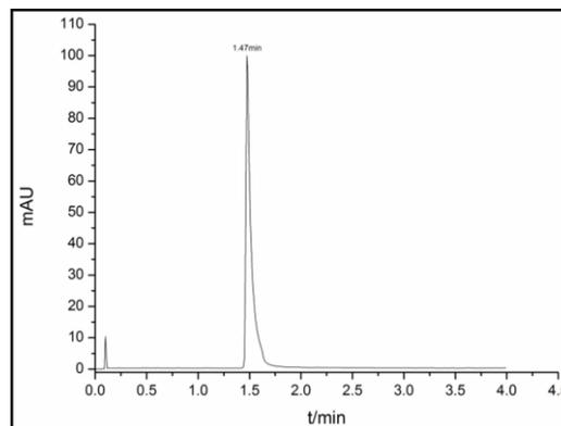
**Fig. 6:** Chromatogram of difenoconazole standard solution
