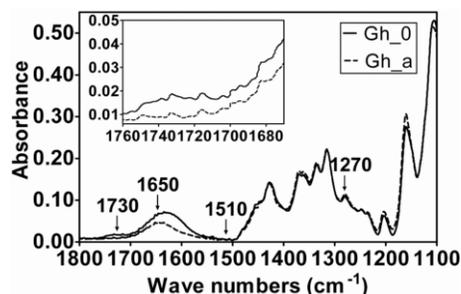
**Fig. 2:** FTIR spectra of cotton fibers. The solid line is the spectrum of washed and cut cotton fiber, and the dashed line is cotton fiber residues after thioglycolate extraction. Values are means of 30 spectra (n = 10 varieties  $\times$  3 replicates)
