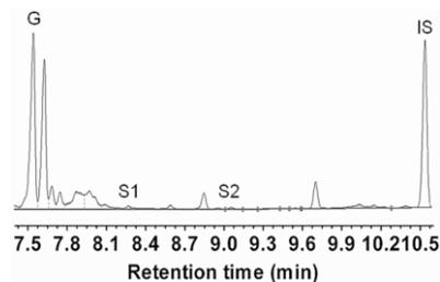
**Fig. 6:** GC chromatograms of DFRC monomers from cotton fiber. G is the coniferyldiacetate monomer from the guaiacyl unit. S1 and S2 are sinapyldiacetate monomers from the syringyl unit. IS is the internal standard (tetracosane)
