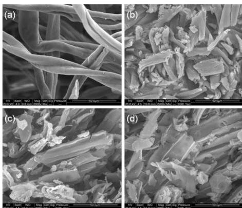
**Fig. 3:** Scanning electron microscopy observation of the cell wall treated by TGA. **a:** Cut mature cotton fiber; **b:** TGA-treated mature cotton fiber; **c:** Milled powder of pine wood; **d:** TGA-treated milled powder of pine wood. Bar = 50.0  $\mu$ m
