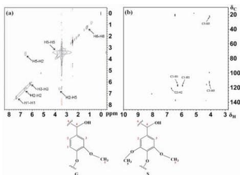
**Fig. 8:** 2D NMR spectrum of phenolics from cotton fiber. **a:** NOESY spectrum; **b:** HMBC spectrum. G is the coniferyl diacetate monomer from the guaiacyl unit. S is sinapyl diacetate monomers from the syringyl unit
