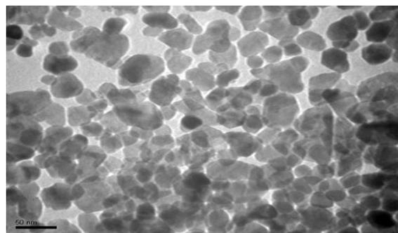
**Fig. 1:** TEM photomicrograph of nano TiO<sub>2</sub>, which shows that the APS is 30±5 nm
