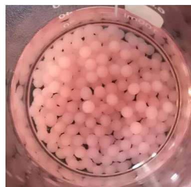
Fig. 1: The immobilization of aspartase cells from Escherichia coli k-12. Sodium alginate ( 25 \text{ g L}^{-1} ), glutaraldehyde ( 1 \text{ g L}^{-1} ) and aspartase cell were mixed in beaker
