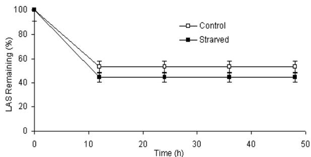
**Fig. 9:** Effect of LAS adaptation on the 300 ppm LAS degradation percentage, the data represent the percentage of degrading LAS expressed as active matter under the same experimental conditions (37°C & agitation rate of 150 rpm), all data are average of three trials with error bars indicating STDEVs ( $\sigma_{n-1}$ )
