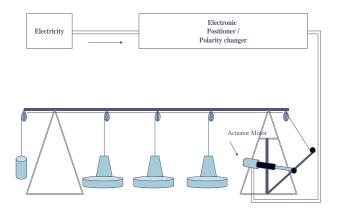
Fig. 1: Automatic feeding system for intermittent feeding
