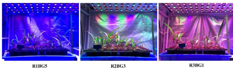
Fig. 1: Layout of the experiment of spectral effect on B. striata seedlings. R1BG5, 13.9% red, 77% green, and 9.2% blue; R2BG3, 26.2% red, 70.2% green, and 3.5% blue; R3BG1, 42.3% red, 57.3% green, and 0.4% blue
