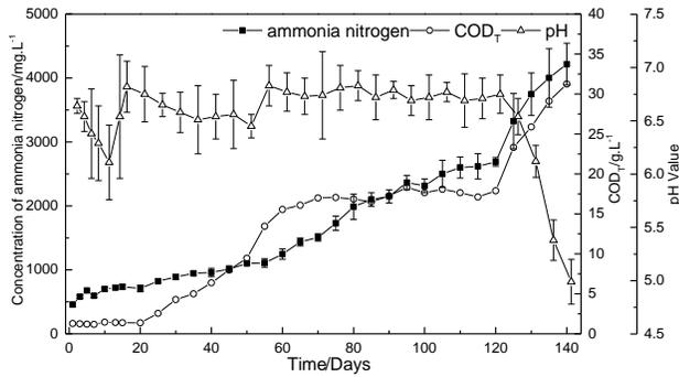
**Fig. 1:** The changes of pH, the ammonia nitrogen and COD<sub>T</sub> concentration in R1 reaction
