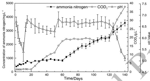
**Fig. 2:** The changes of pH, the ammonia nitrogen and COD<sub>T</sub> concentration in R2 reaction
