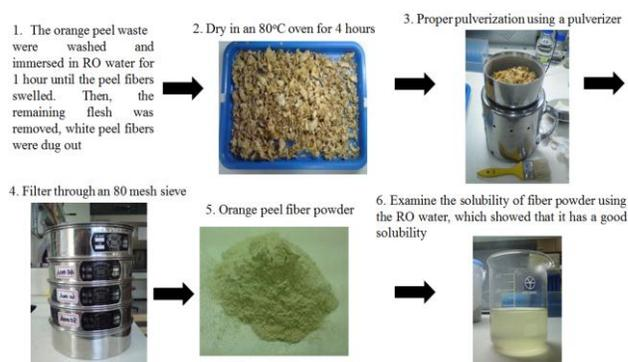
**Fig. 1:** Procedure for preparing OPFP
