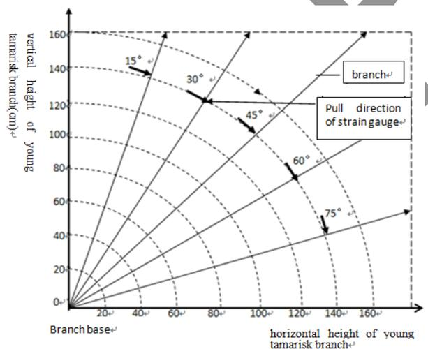
**Fig. 2:** Test model of *T.* resistance measurement
