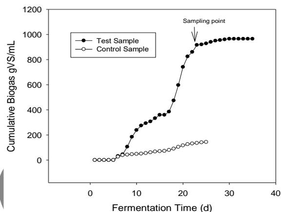
**Fig. 1:** Cumulative Biogas Production
